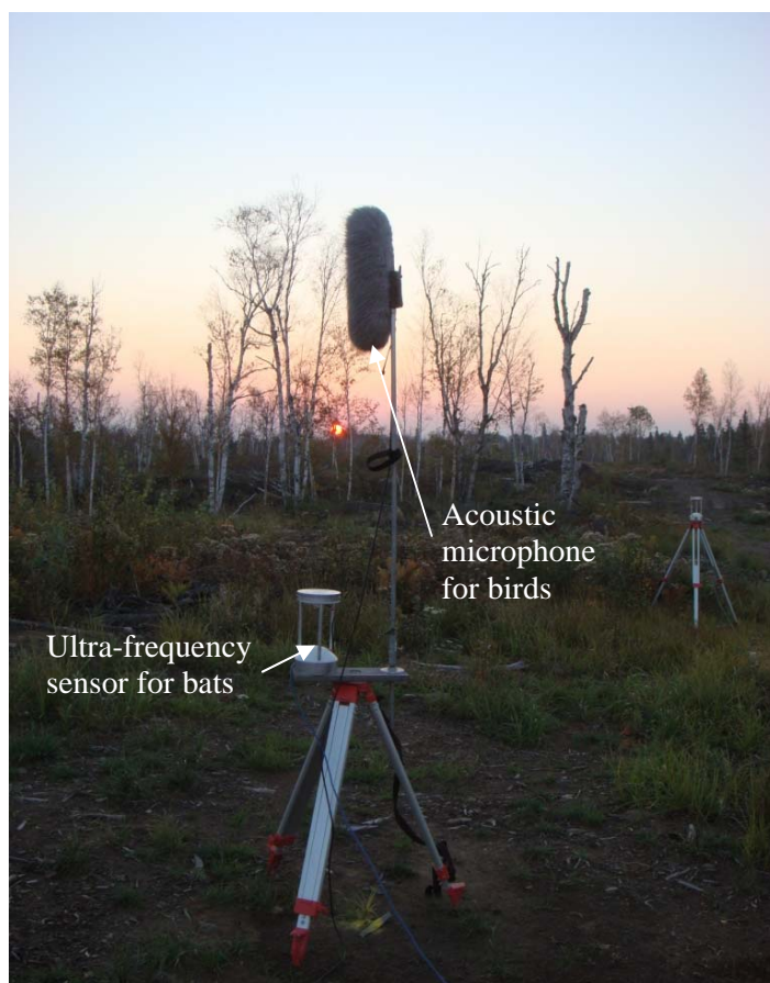
Fig. 2. Acoustic sampling using ultra-frequency sensors bats and acoustic microphones for birds.
